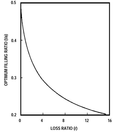
**Fig. 6** Optimum filling ratio vs. loss ratio, twin-slab phase shifter
