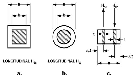
**Fig. 1** Cross sections of waveguide phase shifters.
