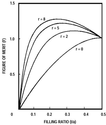
**Fig. 3** Figure of merit vs. filling ratio, twin-slab phase shifter
