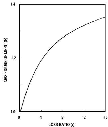
**Fig. 7** Maximum figure of merit vs. loss ratio, twin-slab phase shifter
