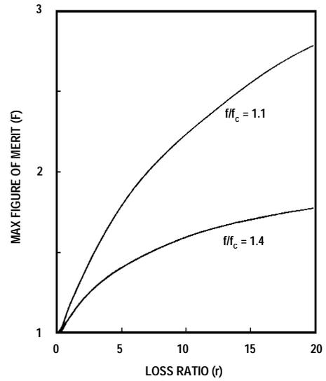
**Fig. 5** Maximum figure of merit vs. loss ratio, square Faraday rotator
