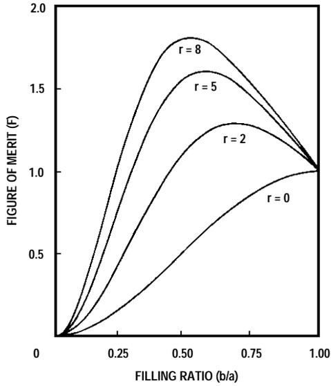
**Fig. 2** Figure of merit vs. filling ratio, square Faraday rotator ( $f/f_c = 1.2$ )
