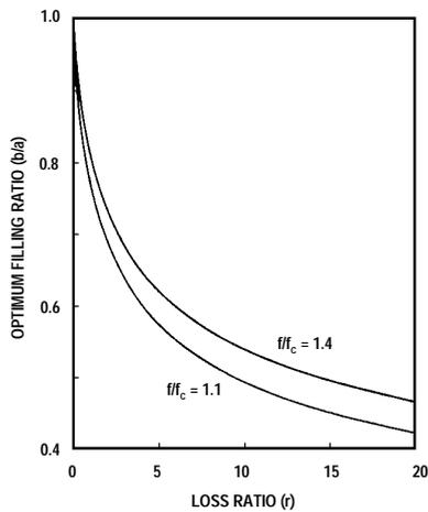
**Fig. 4** Optimum filling ratio vs. loss ratio, square Faraday rotator
