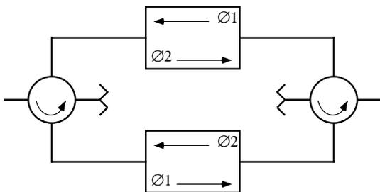
Fig. 1: Basic concept – dual channel phaser
