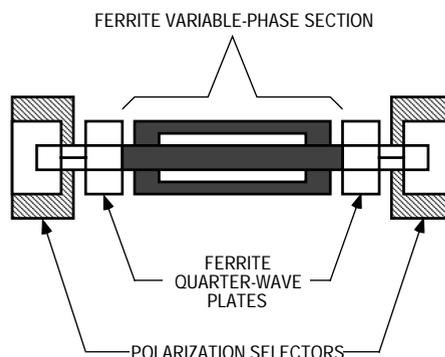
Fig. 2: Phase shifter configuration
