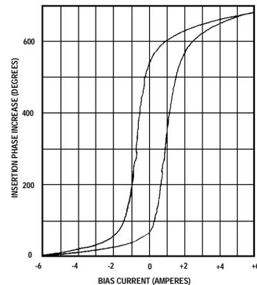
Fig. 6: Phase shift vs. current characteristic
