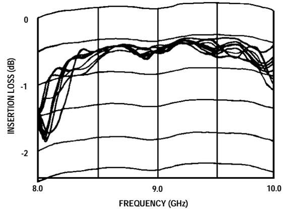
Fig. 4: Insertion loss at random phase states
