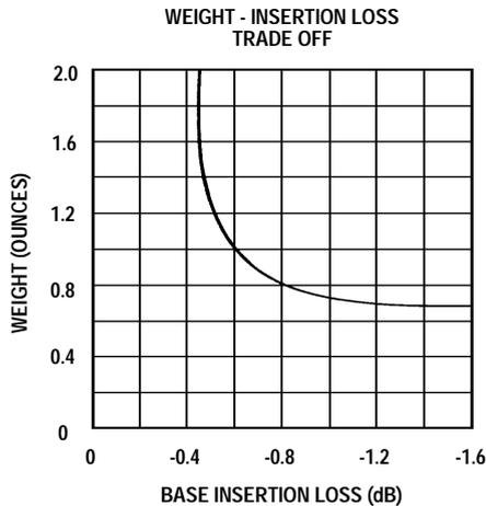
**Fig. 7:** Computed interdependence between minimum weight and insertion loss.
