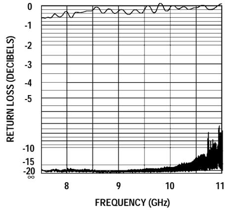
**Fig. 2:** Return loss trace for a dual-mode phase shifter with broad-band matching.
